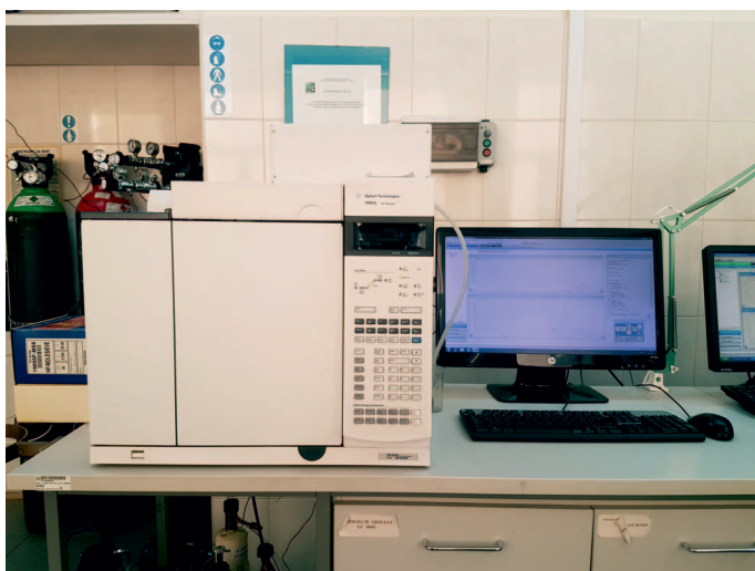
Fig. 1. Dual-channel, valve gas chromatograph AGILENT 7890A
